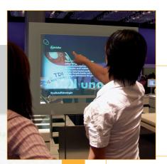
"PointScreen" makes it possible to control the computer intuitively with gestures. The user navigates by merely pointing toward the screen; contrary to touch screen technology, the interaction proceeds completely without touch. The multimedia implementation of screen design and content programming exploits the potential of the interface. Thus the visitor becomes the "conductor" of an audiovisual presentation.
